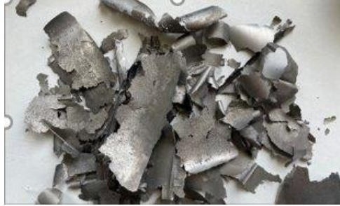
Electrodeposition of Ni-Co alloys on Ti-cathodes after recovery from black mass
