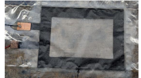
development and testing of HASEL actuator for pressure triggering
