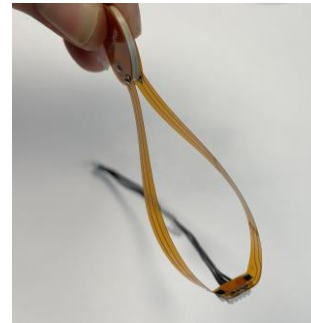
Improved flex-PCB design for ultrasonic sensor, integrating both sender and receiver
